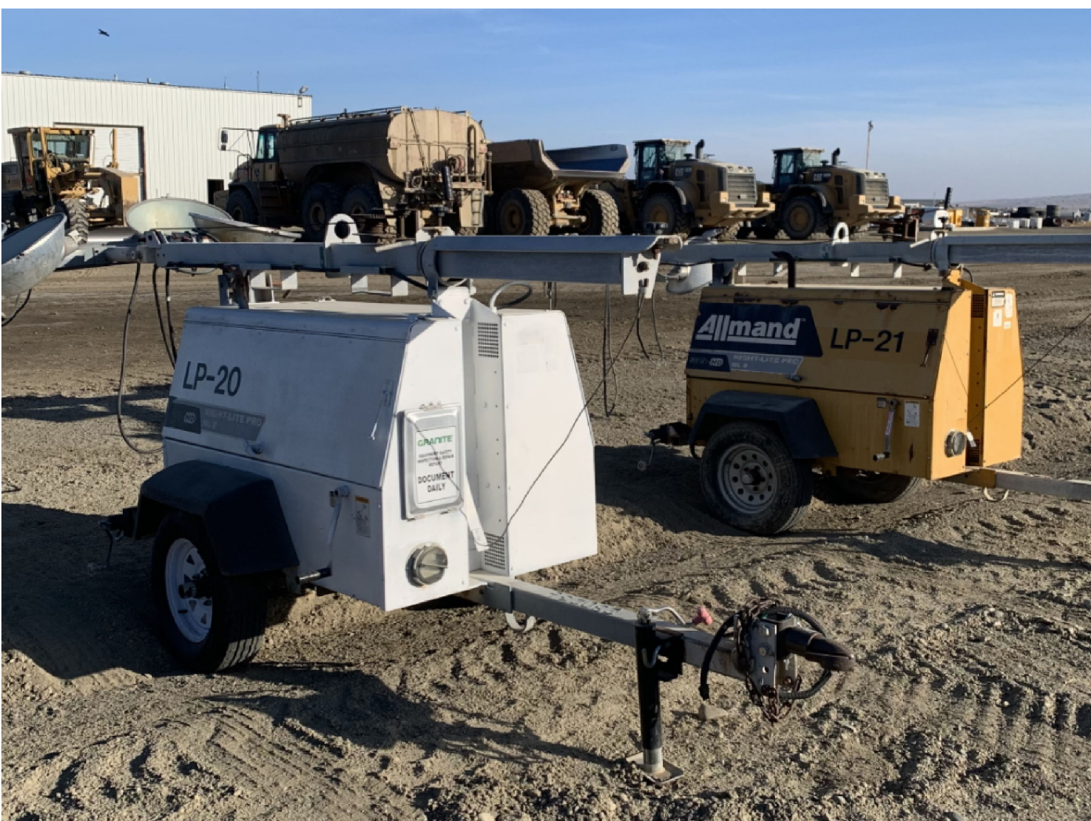
Mining area to be supported by two portable light tower trailers which deploy to 25' - 35' in height and will be used to illuminate operational areas as needed.
