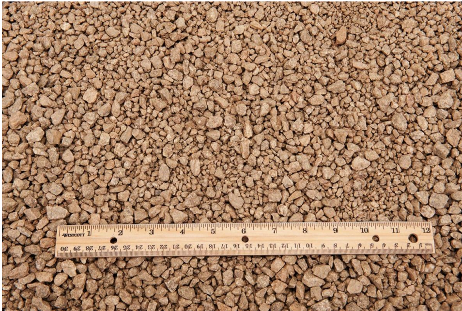
Washed 3/8" "SANTA FE" gravel mulch as supplied by Rosenbalm's Rockery in Fresno, California, or approved equivalent.
