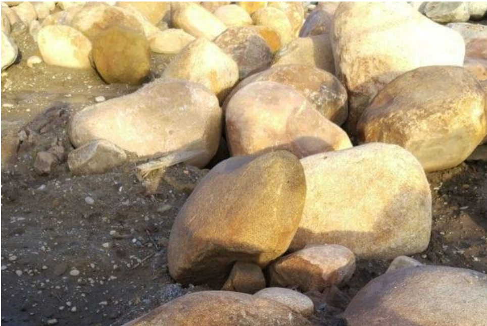
2'-0" to 3'-0" "Mesa Boulder" as supplied by Rosenbalm's Rockery in Fresno, California, or approved equivalent. Boulders are to be an assortment of tan/gold mesa boulders.
