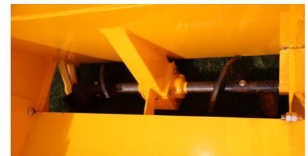
Two (2) 9" Cast Augers are independently operated both Forward & Reverse.
