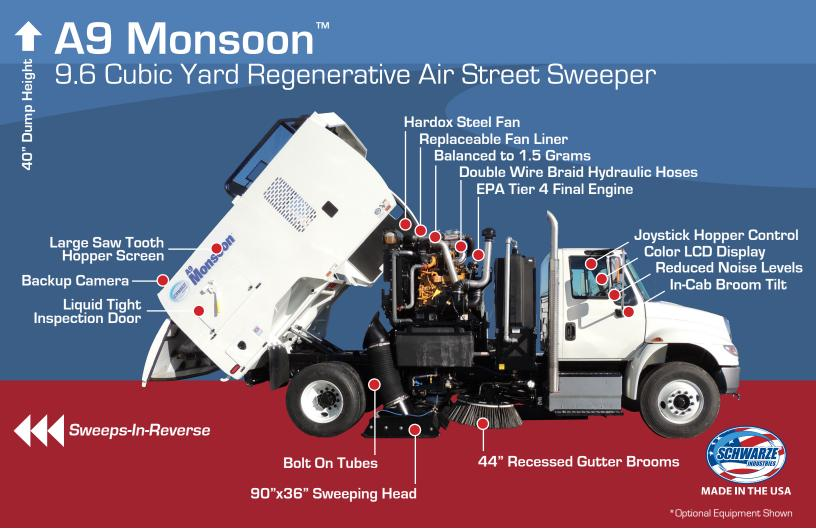
Increased hopper screen surface area through saw-tooth design.
